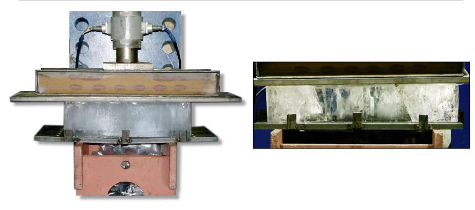
Maximum local ice pressure on side framing stiffeners has been identified by experiment. It was established that design pressure on the plating is 25% less as compared to those specified in current Rules.
